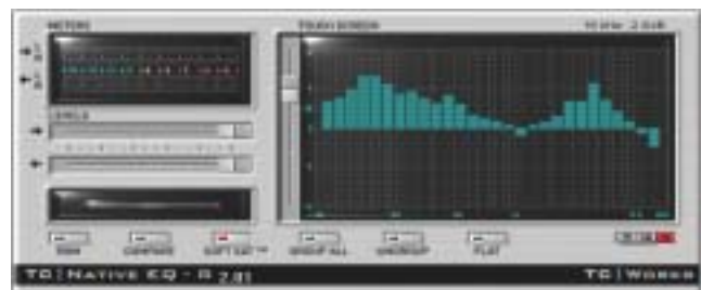
Graphic EQ : bands are fixed, you can only adjust the level of each band.
