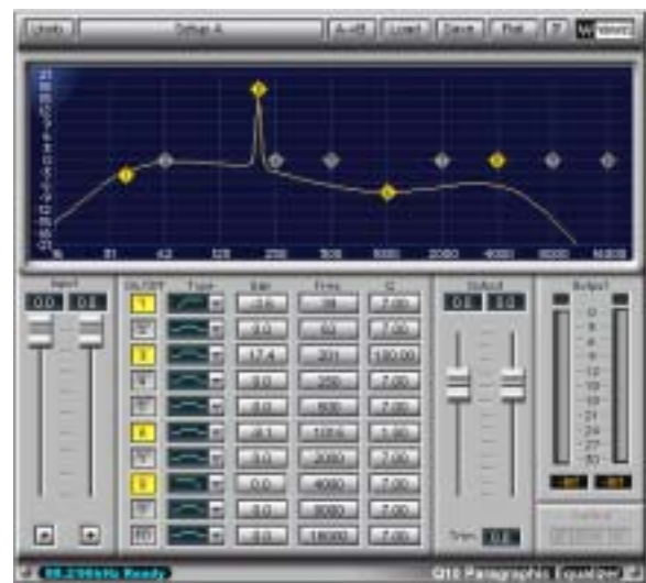
A parametric EQ. From left to right (yellow dots) : hi-pass, bell with high Q value, bell with low Q value, low-pass.
