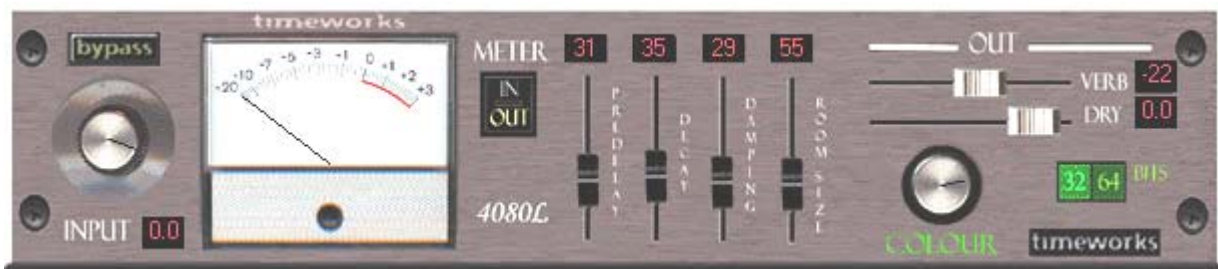
A typical reverb : you can see the predelay, the decay, the damping. In the upper right corner are the Dry/Wet sliders.
